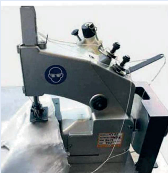
Chain stitch sewing machine 1 needle, 1 thread or 2 needles, 2 threads.
