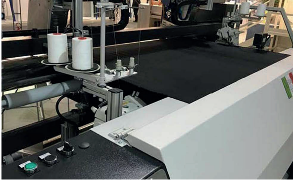
Overlock sewing station or fringed trimmed, speed up to 24 mt/min.
